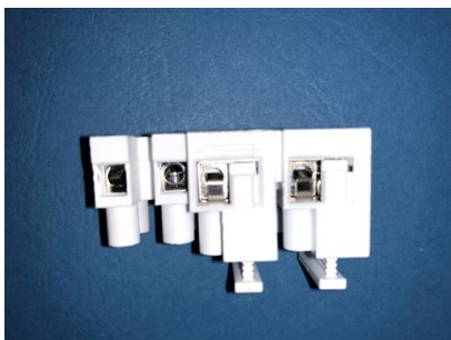
Terminals on the right have compression plates which allow the safe use of multiple conductors.
