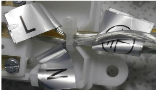
Individual cable cores marked with L, N, and earth symbol
