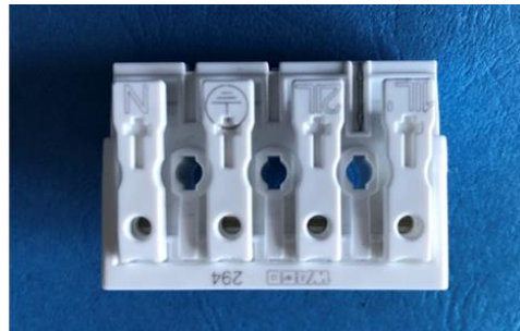
Terminal block with screwless earth connection – the earth connection is made by clipping the terminal block into a pre punched hole in a metal
