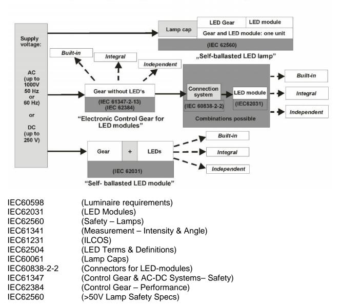
Overview of systems composed of LED modules and control gear
