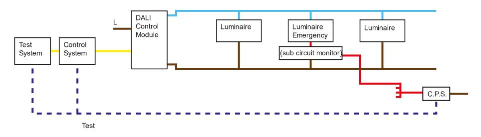
The use of a 'Test' link ensures status sharing between Control, Emergency Test, and Central Power Systems allowing full load testing the
