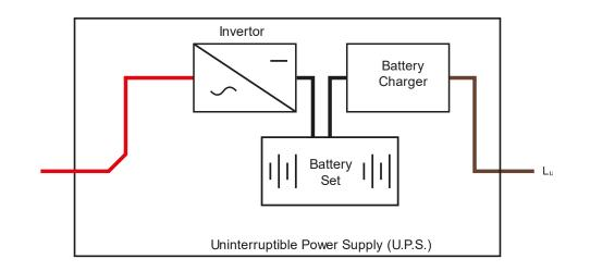
\* Note - UPS Systems are not usually rated correctly or suited to the needs Emergency Lighting. Check for compliance to <u>BS EN 50171:2001 Central Safety Power Supply Systems</u>
