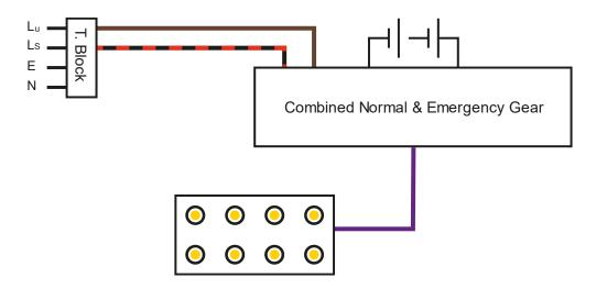
In this instance a single unit of control gear houses components for both normal (mains lighting) functionality and Emergency functionality
