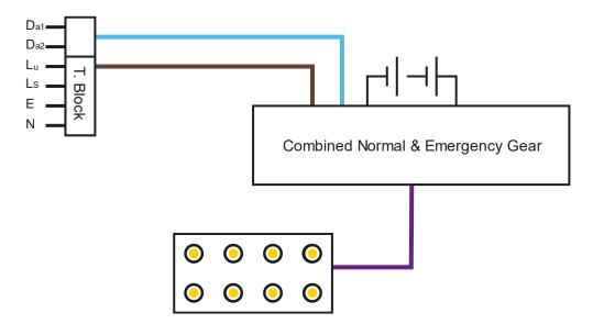
In this instance a single unit of control gear houses components for both normal (mains lighting) functionality and Emergency functionality. In DALI terms it has only one address and is known as DALI Combined Control Gear (which differs from the BS EN 60598 description stated on pages 20 & 21)
