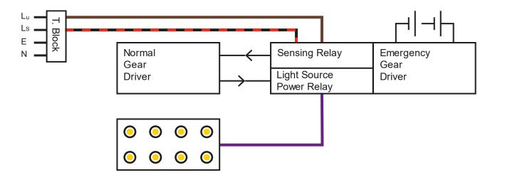
• Maintained: luminaire in which emergency lighting lamps are energized at all times when normal or emergency lighting is required
