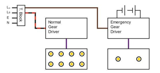
• **Maintained:** a luminaire that also lights at other times (ie is used for both normal lighting and emergency lighting conditions)
