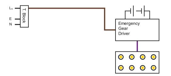
• Non-Maintained : luminaire in which the emergency lighting lamps are in operation only when the supply to the normal lighting fails
